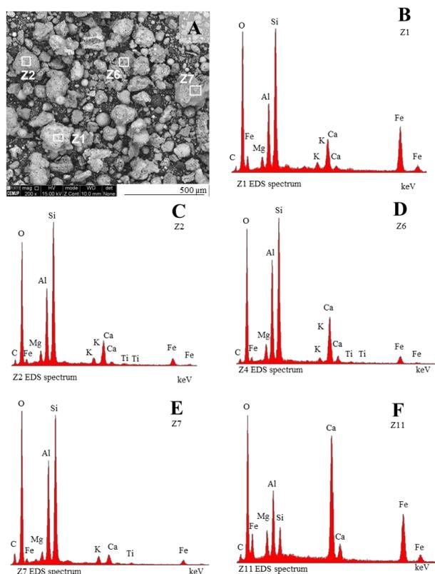
Fig. 5 SEM/EDS analysis of the bottom ash separated using a ferrite hand magnet (Sample MS1; backscattered electron mode).
