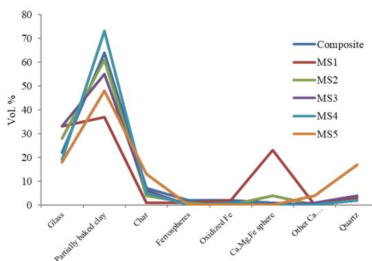
Fig. 4 Petrographic results: distribution of the different morphotypes in the magnetic and non-magnetic fractions.
