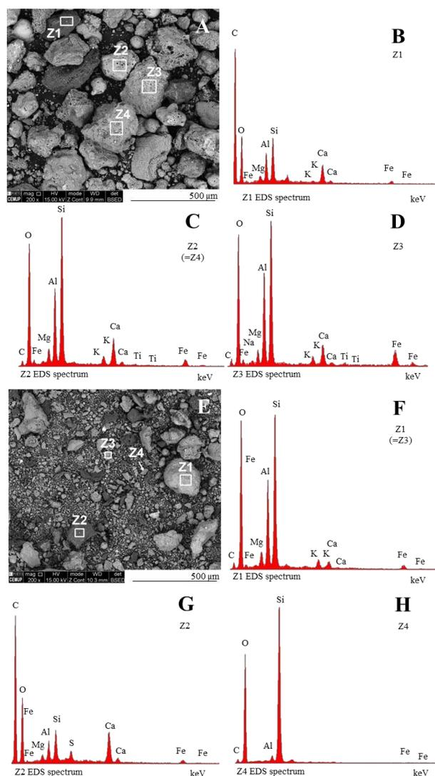
Fig. 7 SEM/EDS analysis of the bottom ash (backscattered electron mode): A to D) fraction separated using Stearns magnetic separator at 18000 Gauss (Sample MS4); E to H) non-magnetic fraction (Sample MS5).
